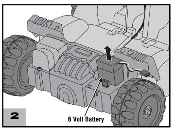
• Lift to remove the battery from the battery compartment.
